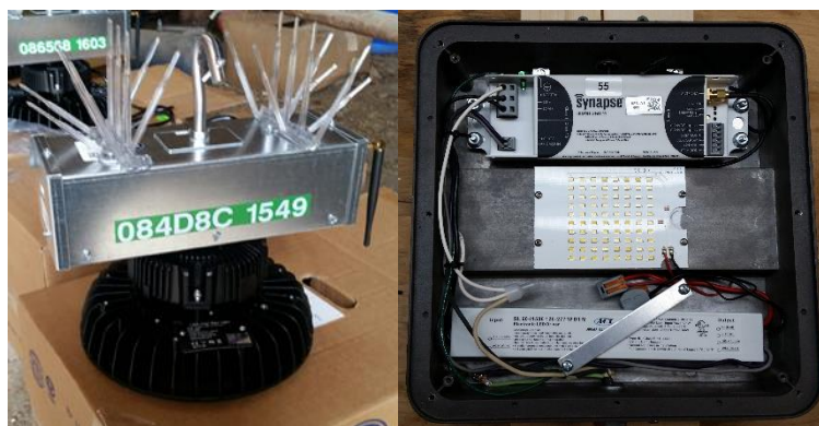
Figure 1. Left: dimmable high bay luminaire with weatherproof box, bird spikes, and antenna; Right: inside of a dimmable canopy luminaire with the DIM10-250 (top) and dimmable driver (bottom)
