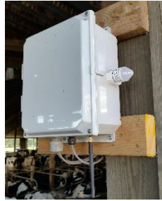
Figure 3. Weatherproof box housing the AIM-121 sensor controller, with side-mounted sensor
