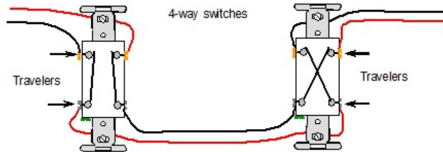
Figure 330.23. Each of these 4-way switches shows a different internal connection. The travelers of each 4-way switch would connect to the traveler terminals of a 3-way switch not shown in this illustration.
