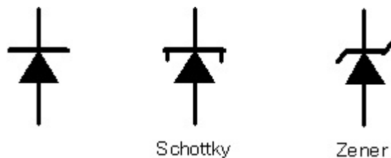
Figure 520.6 The symbol on the left is for a PN junction diode, the one in the middle is a Schottky diode and the one on the right is a zener diode.
