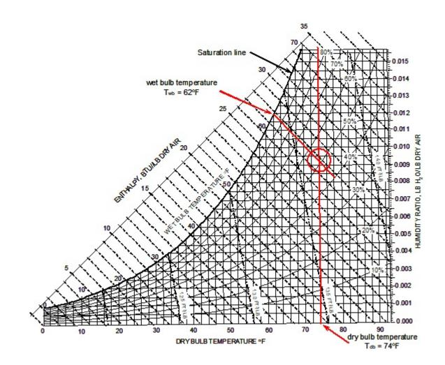
*Figure 386.2* The point that describes the air is found where the vertical line for the dry bulb temperature crosses the diagonal dashed constant enthalpy line that passes through the wet bulb temperature found on the saturation line.
