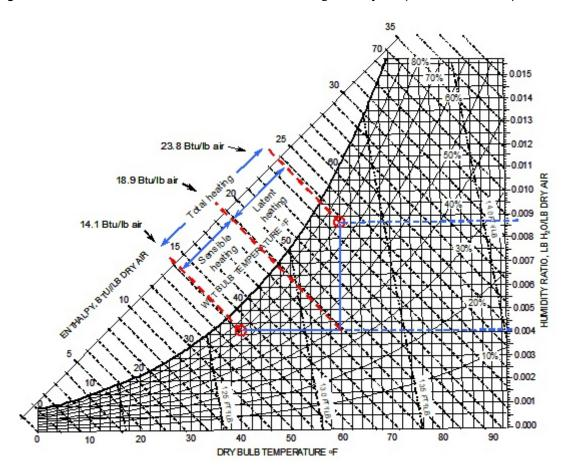
**Figure 386.4** The total heat content of the air leaving a confined space as compared to the air entering the confined space can be subdivided into sensible heat change resulting in a temperature change with no change in water content, and a latent heat change which results in a change in water content at a constant temperature.
