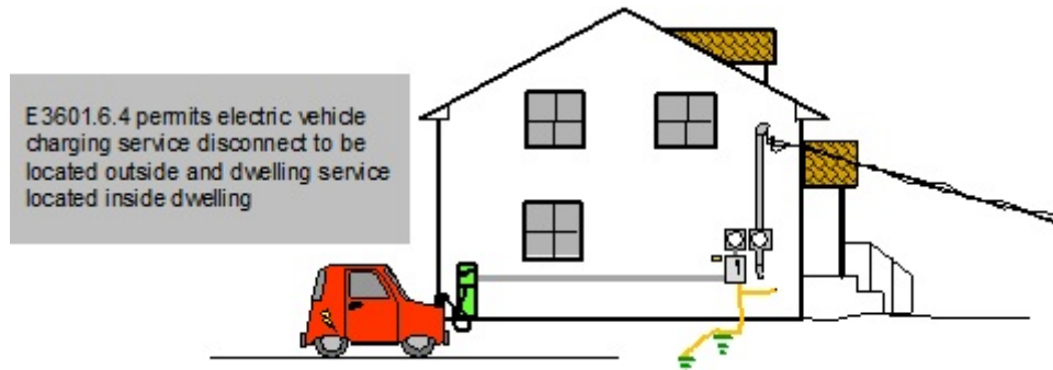
Figure 9 In the case of a one-family or two-family dwelling, it is permitted to provide a separate disconnecting means on the outside of the dwelling for a separately metered electric vehicle charging station service disconnect, but a grounding electrode system is also required.
