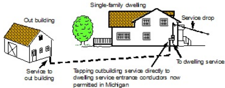
Figure 4. It is now permitted to directly supply an outbuilding from a single-family dwelling service drop or lateral.
