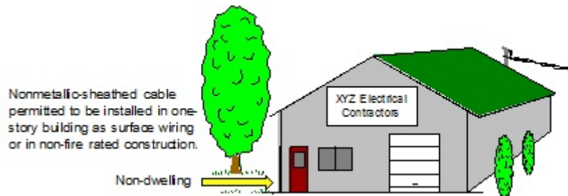
Figure 2. Nonmetallic-Sheathed Cable is permitted to be installed as surface wiring or concealed except for buildings of two or more floors and then it must be installed concealed within walls, floors, or ceilings with a 15-minute finish fire rating.
