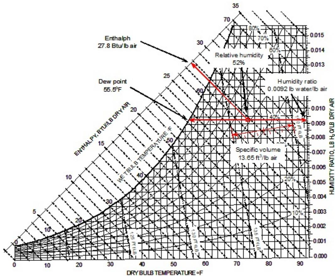
**Figure 386.3** The conditions described by the psychrometer of Figure 386.1 are shown on the chart with the characteristics of the air also shown for those conditions.
