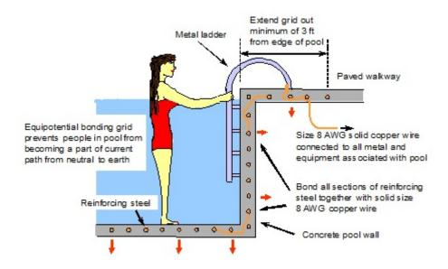
**Figure 3.** Metal steel reinforcing installed in swimming pool concrete walls and floor forms an equipotential grid that prevents a person in the pool from becoming part of a neutral-to-earth voltage circuit.
