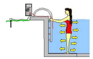
**Figure 1.** When standing in the water of a swimming pool and making contact with a metal object such as a ladder, a person can become a part of a neutral-to-earth voltage circuit and receive a milk shock.
