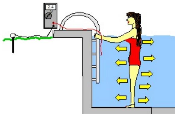
**Figure 1.** When standing in the water of a swimming pool and making contact with a metal object such as a ladder, a person can become a part of a neutral-to-earth voltage circuit and receive a mild shock.
