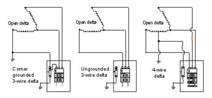
*Figure 8* Open-delta systems can provide 3-wire 3-phase power at 240 volts or at 480 volts cornergrounded or ungrounded. An open-delta 4-wire system can provide single-phase power at 120/240 volts or 3-phase power at 240 volts.
