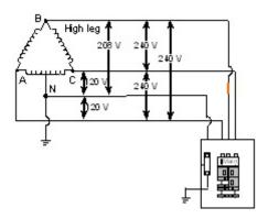
*Figure 7* A 240/120 volt 3-phase, 4-wire system can provide single-phase power at 120/240 volts, or it can provide 3-phase power at 240 volts.
