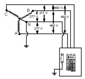
**Figure 5** Common wye 3-phase electrical systems available are 4-wire and may provide power at 208/120 volts or at 480/277 volts.
