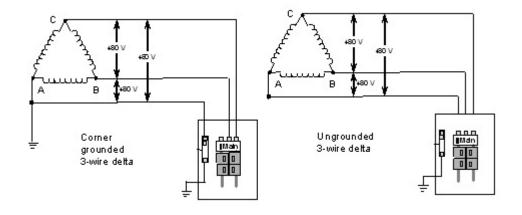
*Figure 6* A 3-wire delta electrical system is available at 240 volts or at 480 volts. One phase conductor may be grounded to form a corner-grounded system.
