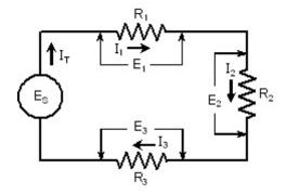
*Figure 10* A series circuit has only one path for current to flow so that the same current flows through every resistor in the circuit.
