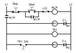
*Figure 15* The four rung ladder control diagram operates two motors using a master control relay, a momentary start-stop push button station, and a time delay relay.
