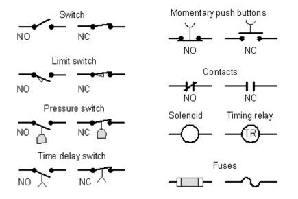
Figure 12 Common control devices found in a motor control ladder diagram.
