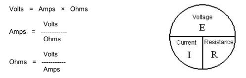
**Figure 1** A circle with voltage over amperes and ohms can be used as a handy way to remember the three forms of the Ohm's law equation.
