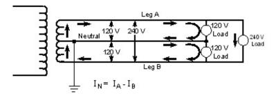
*Figure 4* The current flowing in the neutral of a 120/240 volt 3-wire single-phase system is the difference between the current flowing on the two ungrounded legs.
