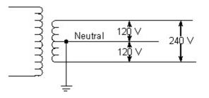
Figure 3 A single-phase, 3-wire electrical system provides power at 120/240 volts.
