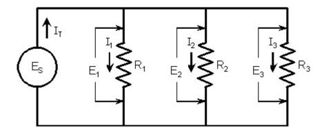
*Figure 11* A parallel circuit is one where current can divide and flow through each element with the total current being the sum of the currents through each resistor.
