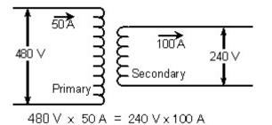
*Figure 2* Volts times amperes on the primary side of a transformer is equal to the volts times the amperes on the secondary side.
