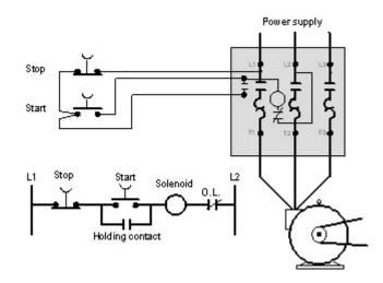
*Figure 14* This control circuit permits the motor to be started or stopped from one location with one push button to start and another push button to stop.
