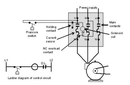
Figure 13 A pressure switch controls a motor using a two-wire control circuit.
