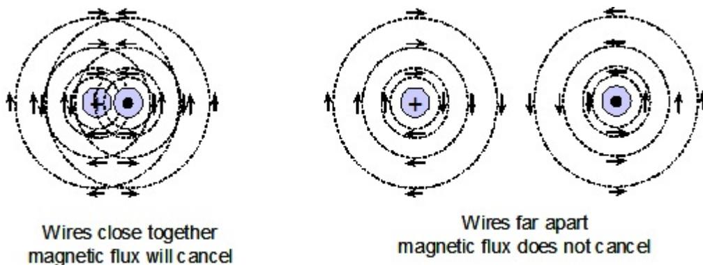
**Figure 229.3** The two small circles at the right are wires of the same circuit carrying the same current, but the flow is in opposite directions. A magnetic flux builds up around each wire but the polarity is opposite so the magnetic flux will cancel if the wires are close to each other as illustrated at the left.
