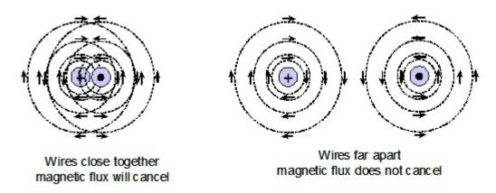
**Figure 229.3** The two small circles at the right are wires of the same circuit carrying the same current, but the flow is in opposite directions. A magnetic flux builds up around each wire but the polarity is opposite so the magnetic flux will cancel if the wires are close to each other as illustrated at the left.
