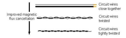
**Figure 229.4** Wires of the same circuit arranged close together will achieve good magnetic flux cancellation, by twisting the pair of wires together achieves even better magnetic flux cancellation.
