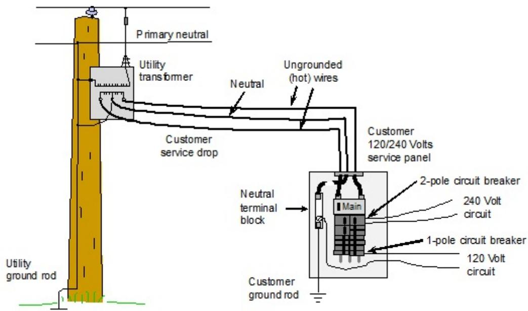
**Figure 219.2** The two ungrounded wires from the utility transformer connect to the main circuit breaker and the neutral conductor connects to the neutral terminal block. A 240 volt circuit originates with a 2-pole circuit breaker, and a 120 volt circuit originates at a 1-pole circuit breaker with the other wire connected to the neutral.
